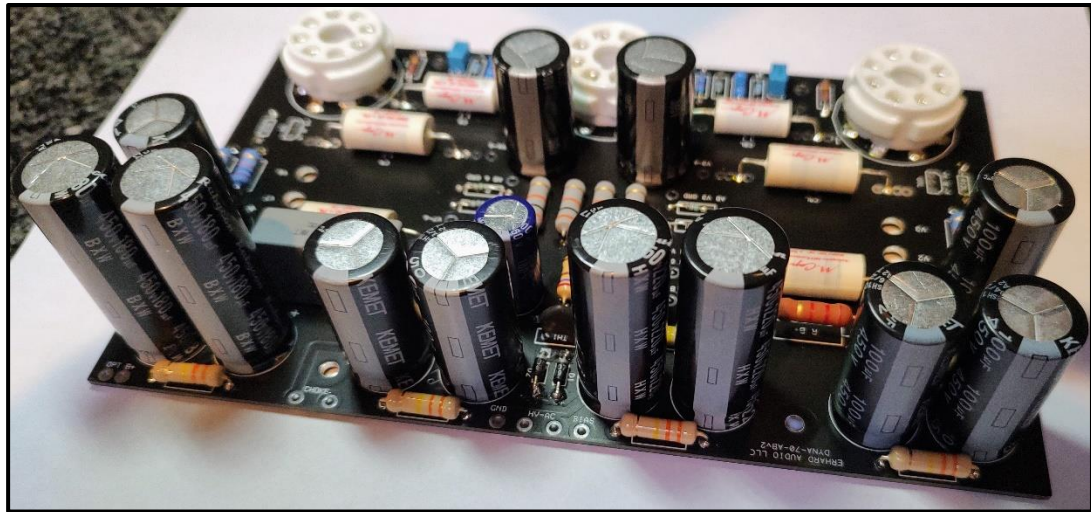
Photo 3: All Electrolytic Cap Cans have the Ground terminal facing the rear of the Circuit Card Assembly
