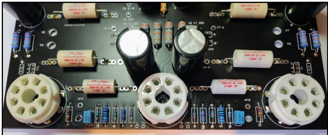
Photo 4: Socket Orientation for 6SN7's is indicated on the PCB
