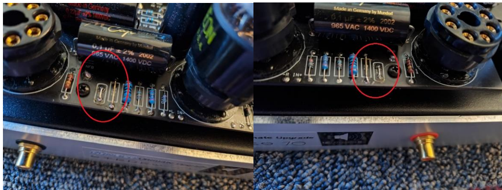
Photo 4: Removal of 16-Ohm NFB Components from Dyna Ultimate Upgrade PCB
