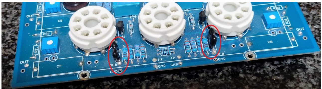
Photo 7: ST-70 / Mk III / Mk IV - Remove R8 & C12 from PCB's
