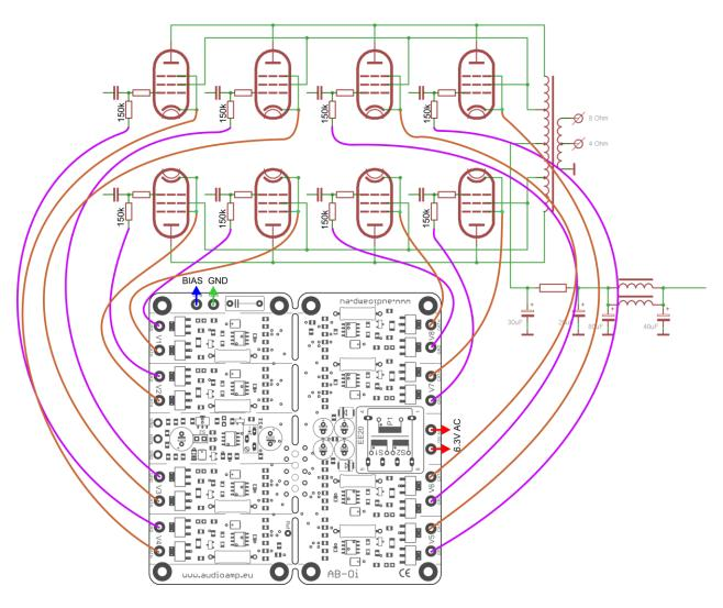
Use this diagram as a reference to the wiring of the AB-Oi module into your amp.
